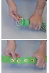
5) Friction and Mating Buckles Inspect the buckle for distortion. The outer bars and center bars must be straight. Pay special attention to corners and attachment points at the center bar.
